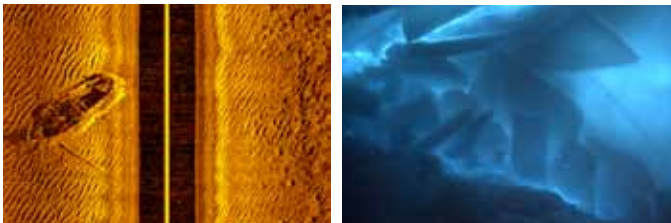
Left: Wreck of a small fishing boat captured on a 900 kHz side scan.
