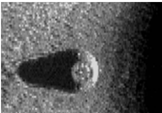
Left: Side scan image of a mine like object captured at 900 kHz.
